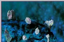
Powdered lead sorbent bonded onto the surface of an activated carbon particle
