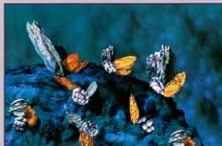
Powdered lead sorbent, antimicrobial, and arsenic reduction compounds bonded onto the surface of an activated carbon particle
